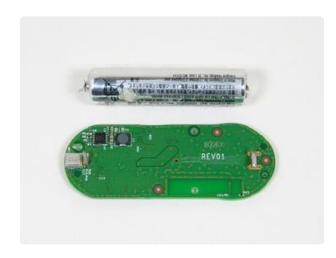
Pull the Dash circuit board out of the case. You will notice on the back of the Dash board a AAA lithium battery is connected. Unfortunately the battery is welded to tabs on the circuit board so it is not a simple process to remove or replace the battery.
